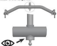
Caution: the axle and the hanger bar must be replaced immediately. The patient lift must not be used until all worn parts have been replaced and a verification has been carried out before putting it back into service.
